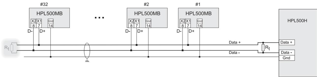
Figure 2. MODbus network with Remote Terminal Unit HPL500H
