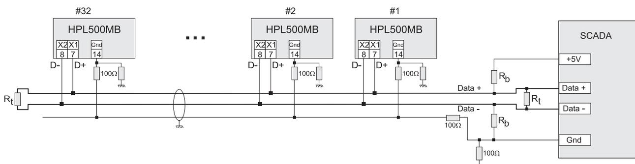
Figure 1. Industrial Modbus network according to EIA485
