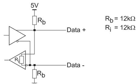
Figure 3. HPL500 input impedance and built-in bias resistors
